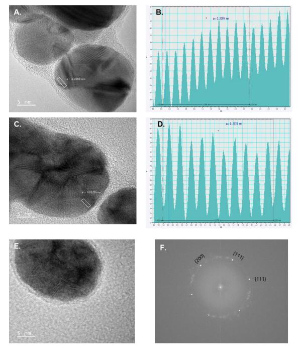
High resolution transmission electron microscope analysis on silver nanoparticles
