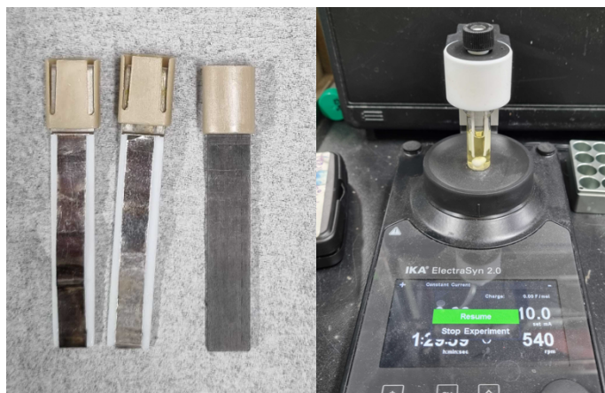
Figure S1. Electrode and Ika electrasyn 2.0 set up. (Pt : 8.00 mm × 52.5 mm × 1.50 mm, graphite : 8.00 mm × 52.5 mm × 2.00 mm)
