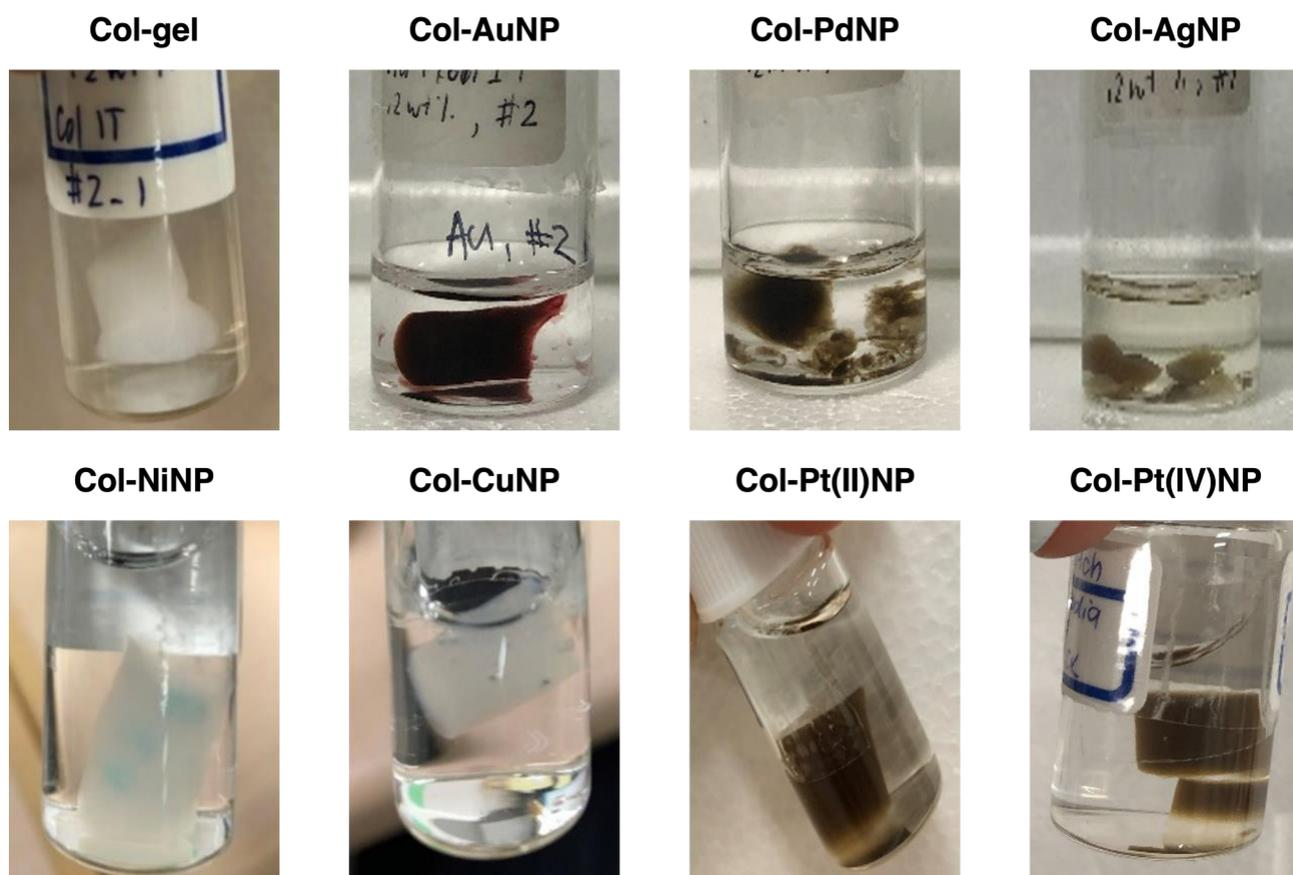
**Figure S1.** Pictures of Col-TMNP hydrogels after  $\gamma$ -ray irradiation
