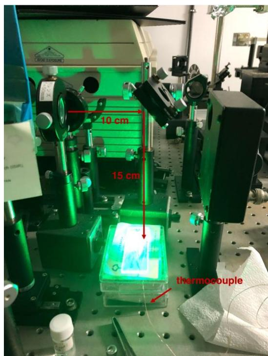
Figure S5. Laser setup for photothermal experiment
