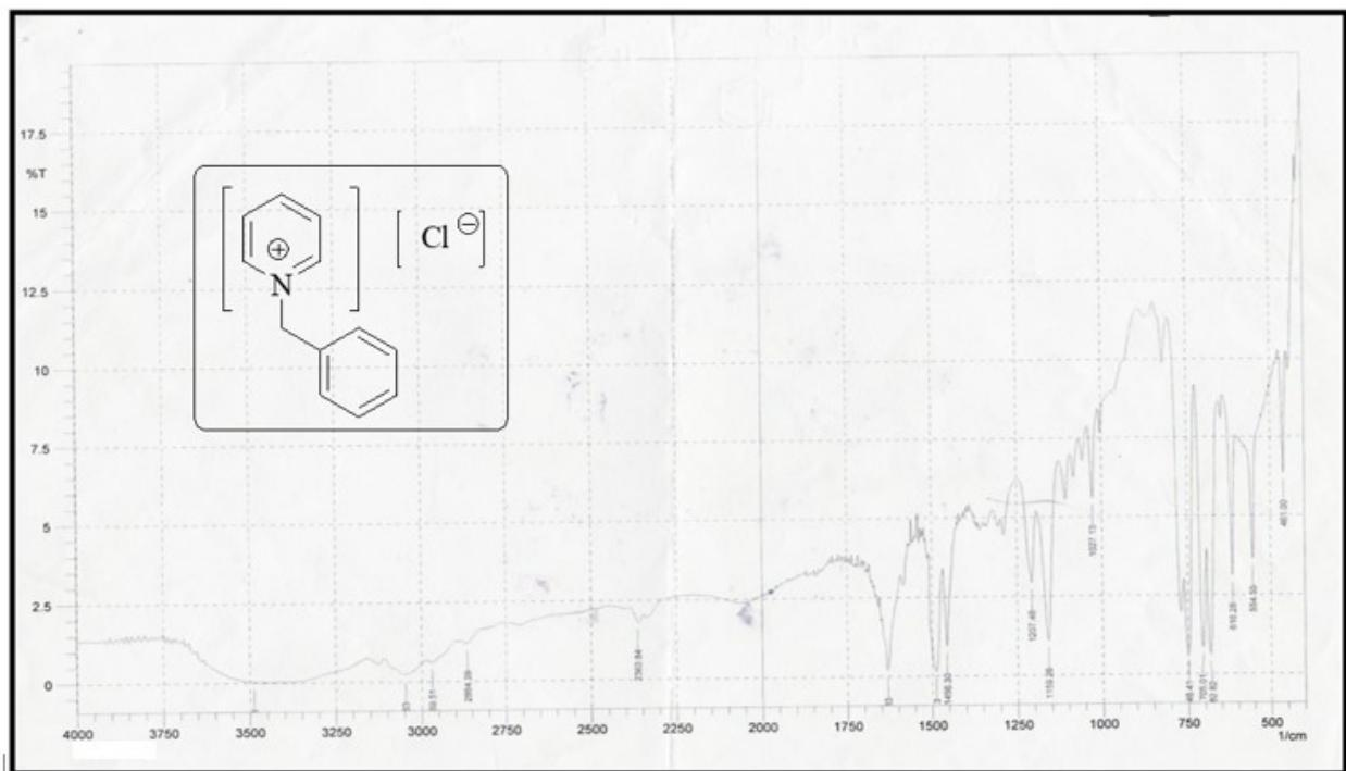
Figure S29: FT-IR spectrum of synthesized ionic liquid of IL-19
