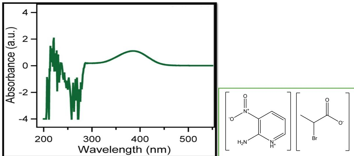
Figure S23: UV-VIS spectrum of synthesized ionic liquid of IL: 18 (385 nm)
