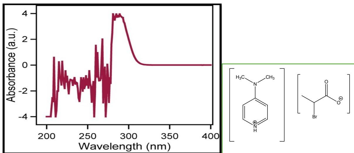
Figure S15: UV-VIS spectrum of synthesized ionic liquid of IL: 12 (285 nm)
