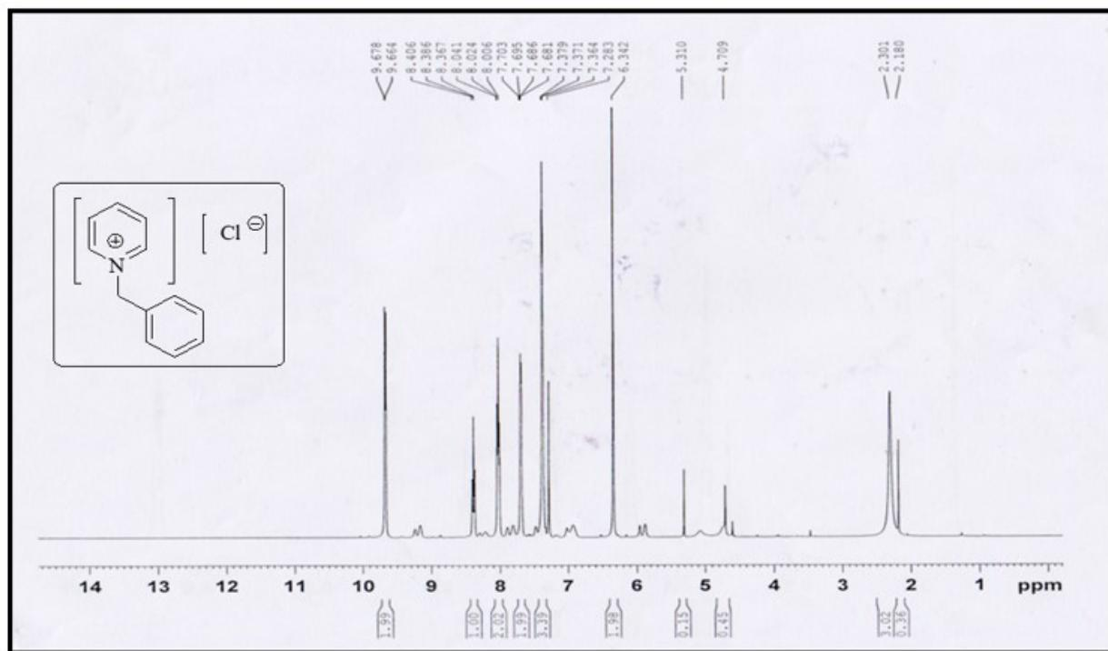
Figure S30: <sup>1</sup>H-NMR spectrum of synthesized ionic liquid IL-19
