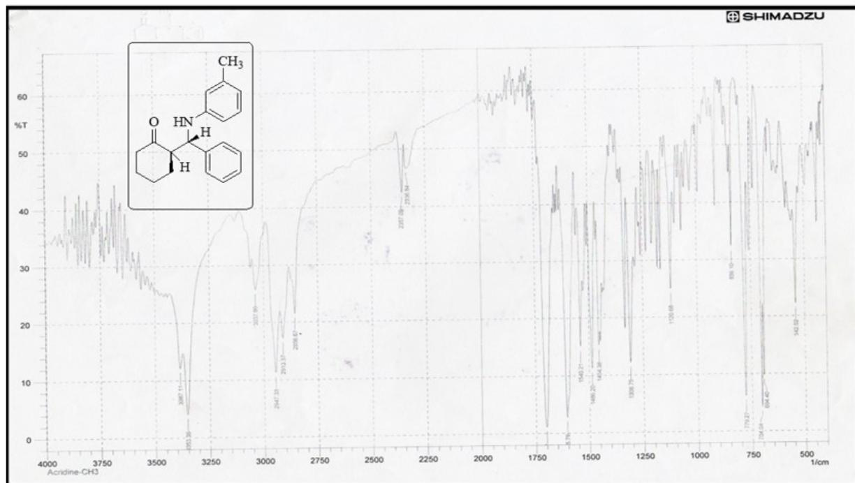
Figure S33: FT-IR spectrum of synthesized Mannich Base Compound MB:01
