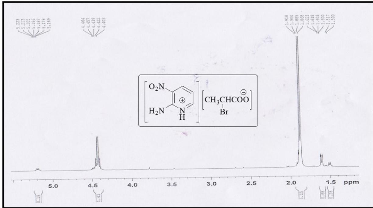
Figure S26: <sup>1</sup>H-NMR spectrum of synthesized ionic liquid of IL: 18
