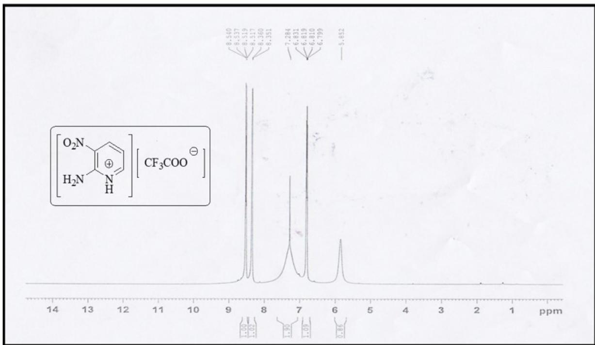
Figure S21:  ${}^1\text{H}$ -NMR spectrum of synthesized ionic liquid of IL: 17
