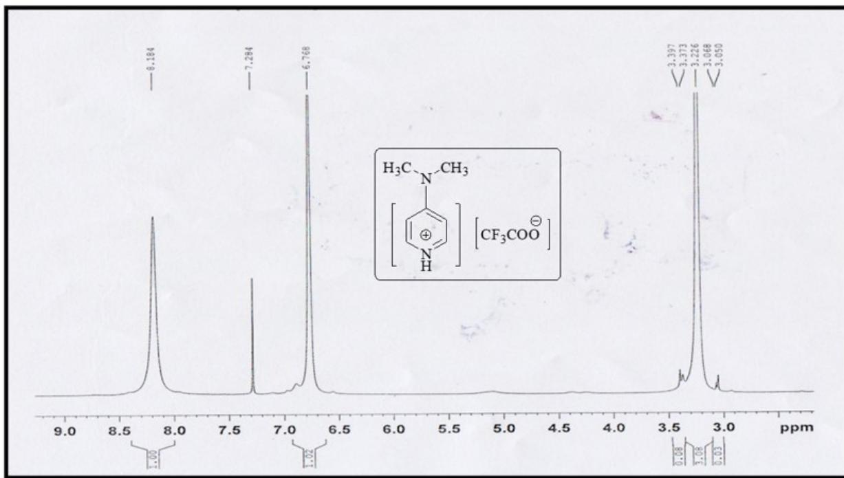
Figure S14: <sup>1</sup>H-NMR spectrum of synthesized ionic liquid of IL: 11
