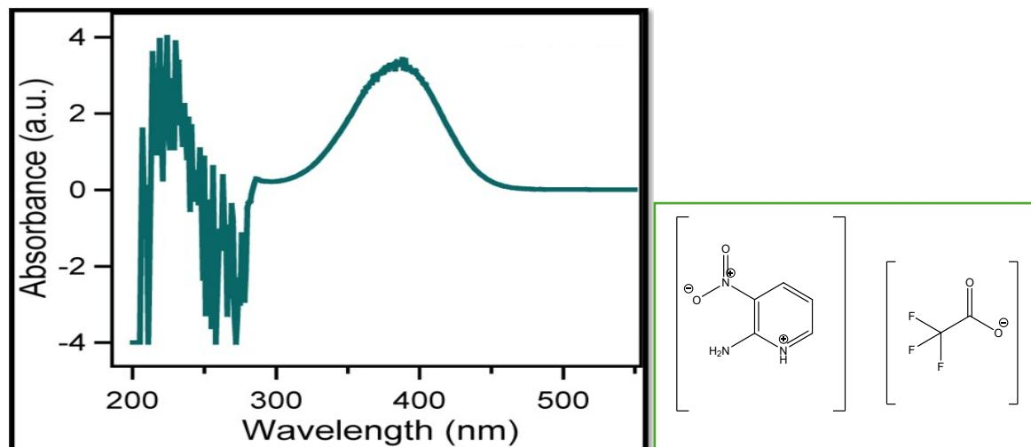
Figure S19: UV-VIS spectrum of synthesized ionic liquid of IL: 17 (389 nm)
