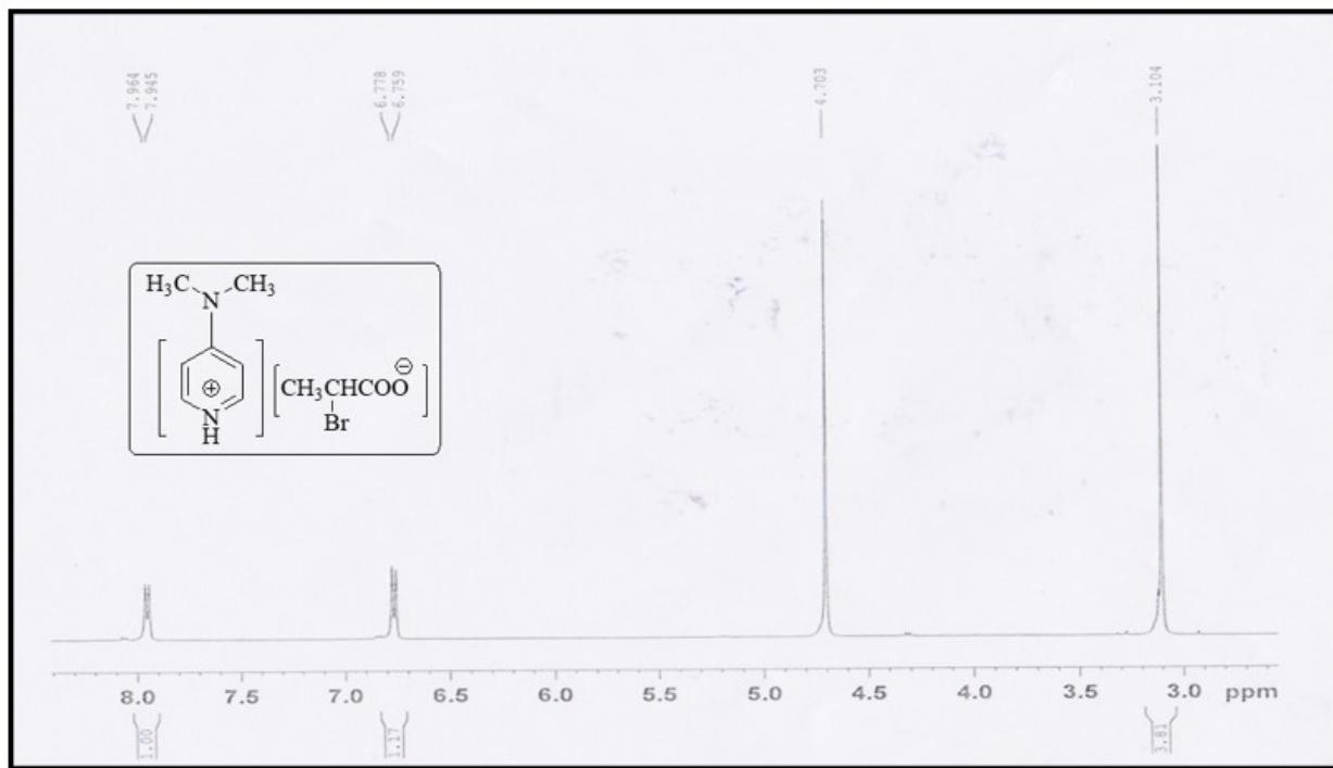
Figure S18: <sup>1</sup>H-NMR spectrum of synthesized ionic liquid of IL: 12
