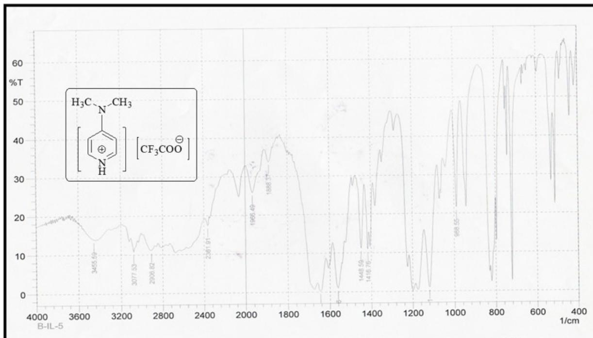
Figure S12: FT-IR spectrum of synthesized ionic liquid of IL: 11
