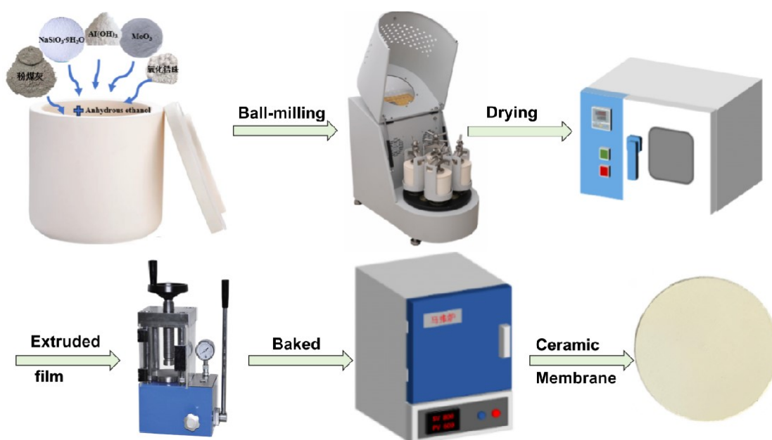
Figure S1. Illustration of the preparing method of the porous ceramic membrane.
