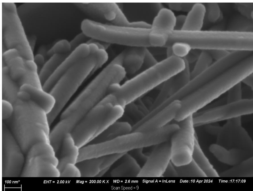
Figure S2: FESEM micrograph of Bi 2 O 2 S
