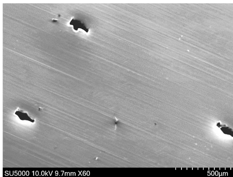
Fig. S1. SEM image, showing the prepared Al electrode by using microneedle roller.
