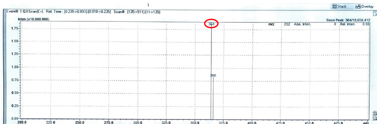
Figure S3. LCMS of ( E )-2-(((4-(dibenzo[b,d]furan-4-yl)phenyl)imino)methyl)phenol ( DBF1 ). [recorded on LCMS-8060NX with heated ESI probe from Shimadzu].
