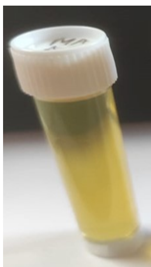
Fig. S1. Colloidal solution of maleic acid functionalised AgNPs.
