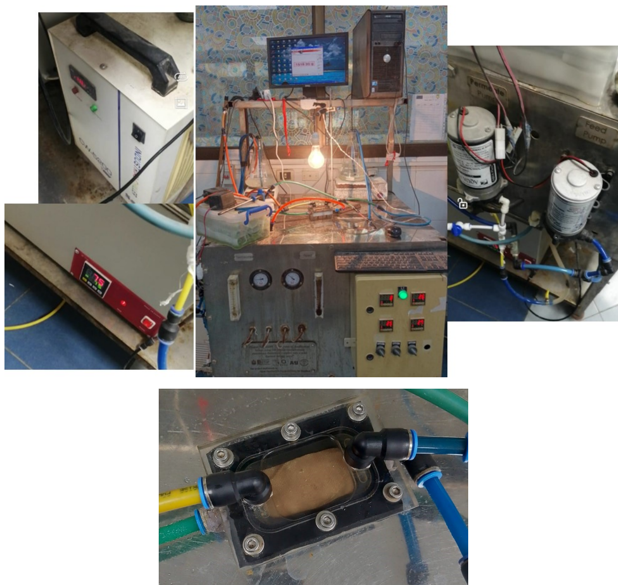
Fig.S1 Real form of the device ,and the used Cell with quartz window.
