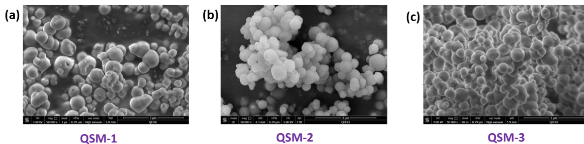
Figure 1. SEM images for silica synthesised using β-CD amount a) 0.3 g, b) 0.65 g, and c) 0.9 g
