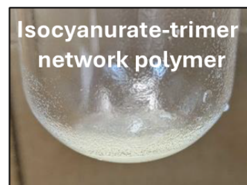
Fig. S29 Reaction of BADGE with HDI leading to formation of a cross-linked isocyanurate polymer, with no cyclic carbamate formation observed.
