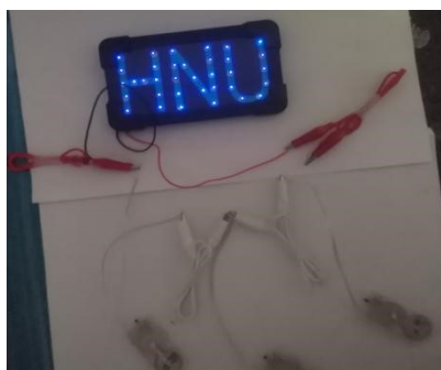
Figure S7. The 1.5V sign can be lit by connecting multiple PPy/GEL SCs in series.
