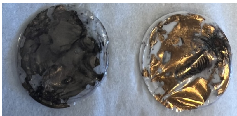
Fig. S 4 Damaged membranes after application of 5V
