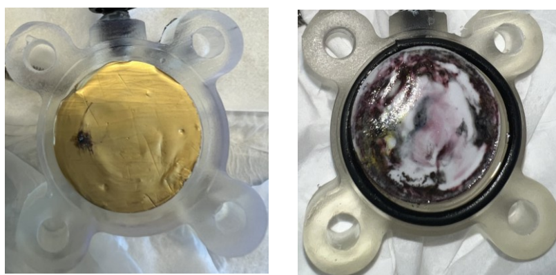
Fig. S 5 Result of high salt buffer runs: Left - burn marks on the gold sputtered membrane-gold pin point of contact due to flow of current Right side - burn marks on affinity membrane.
