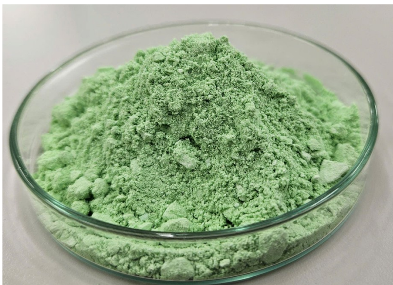
Figure S7. Photograph of the green nickel precipitate obtained under optimal precipitation conditions. The distinctive green color confirms the formation of \text{NiOOH} and \text{Ni}(\text{OH})_2 as the dominant solid phase.
