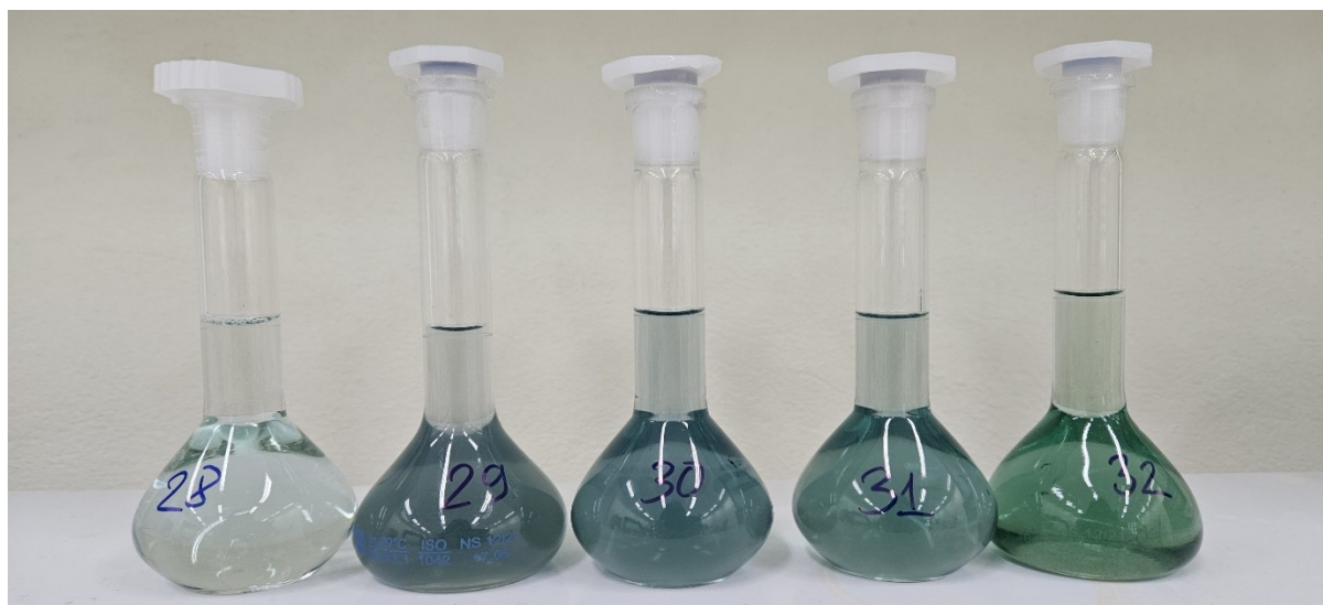
Figure S5. Solution (diluted 100 times) after leaching with \text{H}_2\text{SO}_4 at concentrations of 2 – 5 – 10 – 15 – 20%
