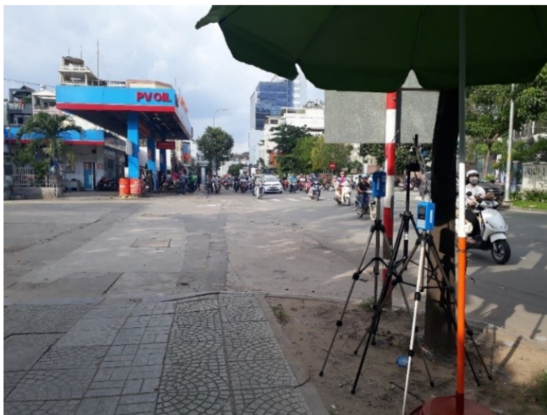
Figure S2 - Field photograph of BTEX concentration monitoring conducted at the fuel station
