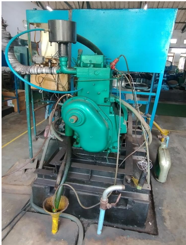
Figure S6. The IC engine (backside view), displaying the fuel injector and air filter.
