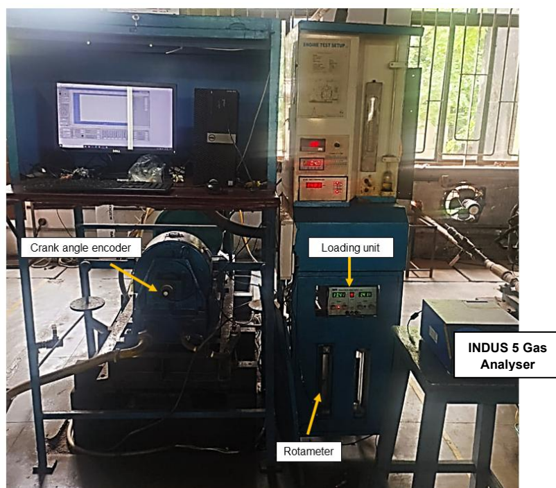
Figure S4. Computerized internal combustion engine experimental test facility (front view).
