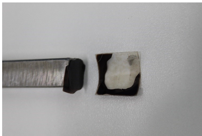
Figure S4. 35 days aged PE-Coated samples after adhesion strength test.
