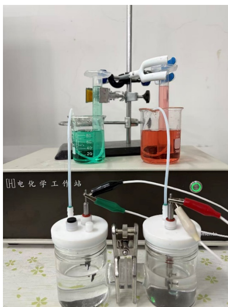
Fig. S7 Schematic diagram of the faradaic efficiency measurement setup
