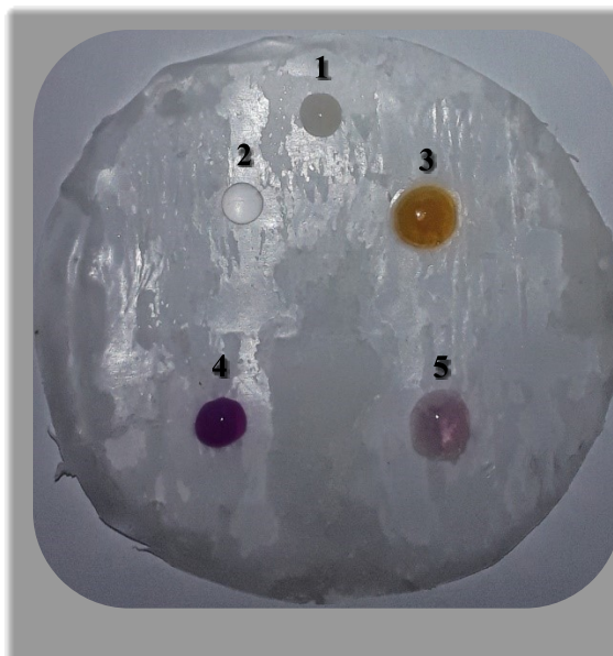
Fig. S1. Photographs of modified PCMA with (1) fish meat, (2) H 2 O, (3) HA/Neocuproine/Cu(II), (4) diphenyl carbazide/H 2 SO 4 /Cr(VI), (5) dimethylglyoxime/Ethanol/NaF/Na 2 S 2 O 3 /Ni(II).
