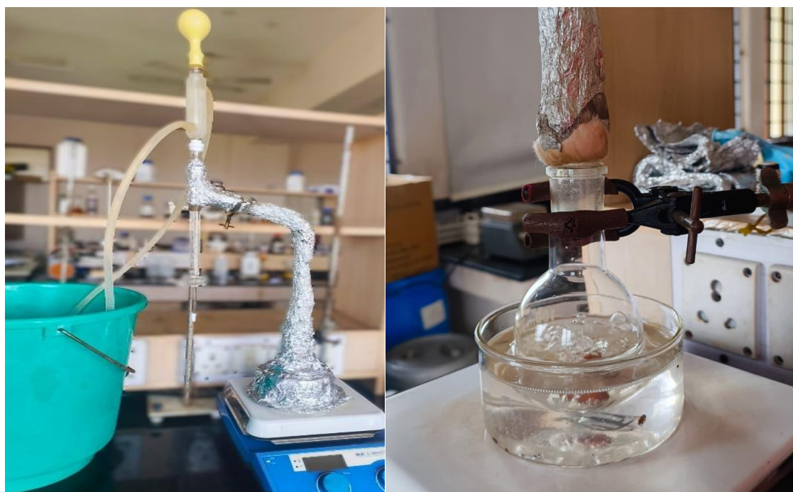
Figure S38. Photographic images of the experimental setup for the acetalization reaction in a Dean-Stark apparatus.
