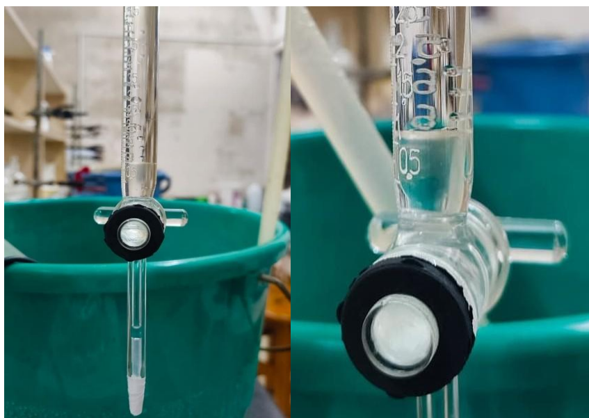
Figure S37. Photographic image of the separated water by azeotropic distillation of cyclohexane in the Dean-Stark apparatus.
