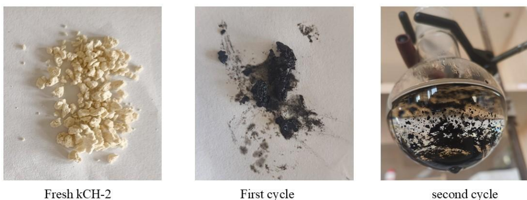
Figure S32. Photographic images of the kCH-2 catalyst isolated from the reaction mixture after each catalytic cycle.
