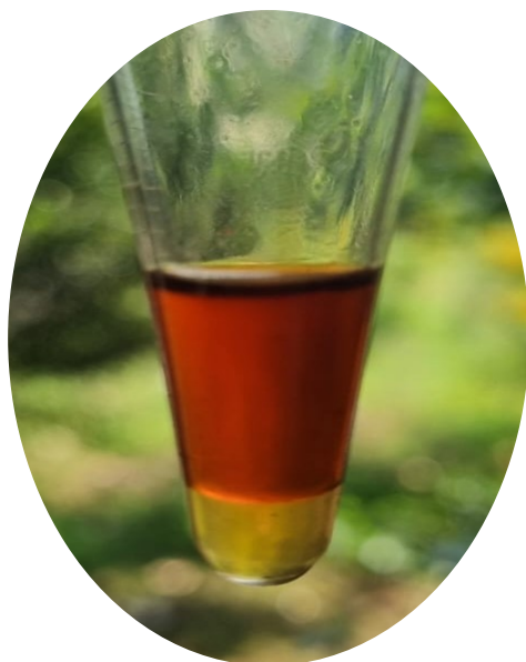
Fig. S1. Purified biofuel fraction, isolated through fractional distillation based on boiling point differences (40 – 60 °C).
