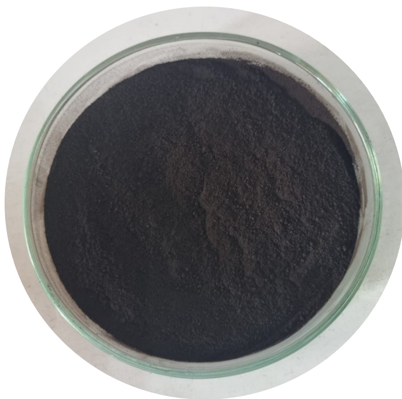
Fig. S3. Biochar, synthesized at 550 °C via pyrolysis of fleshing waste.
