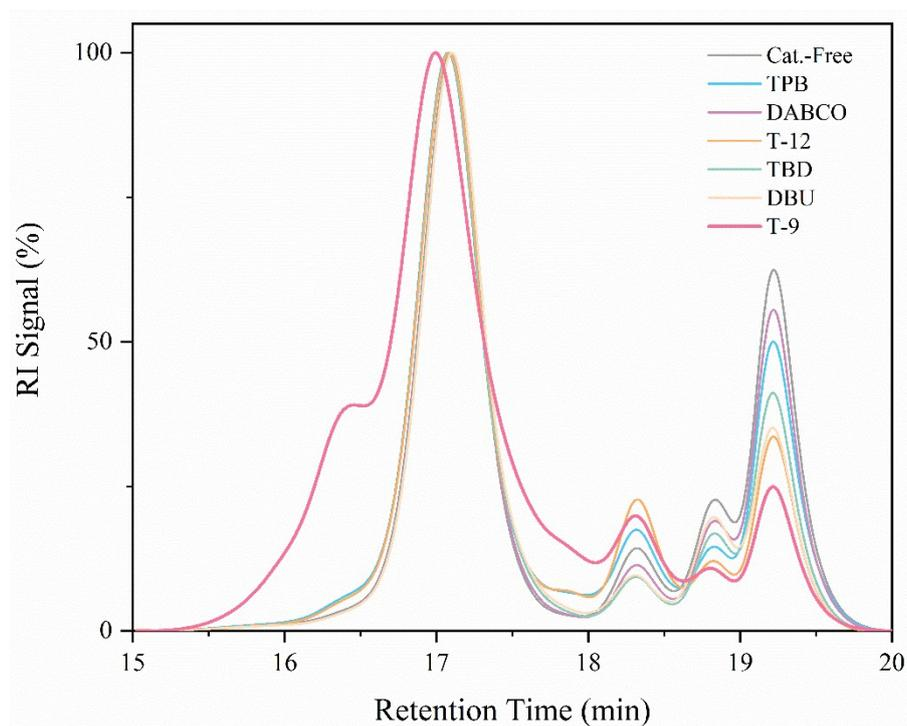
Fig. S3 The GPC curve of polyurethane prepolymer prepared under different kinds of catalysts
