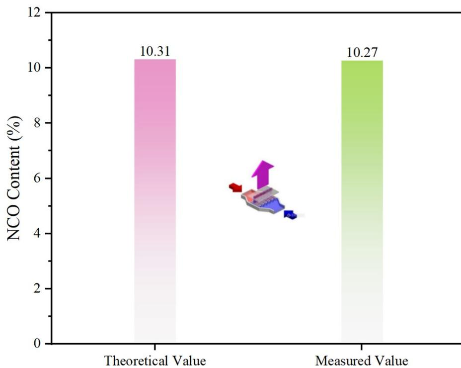
Fig. S1 Comparison of theoretical value and test value of -NCO content in the mixture at the outlet of micromixer.
