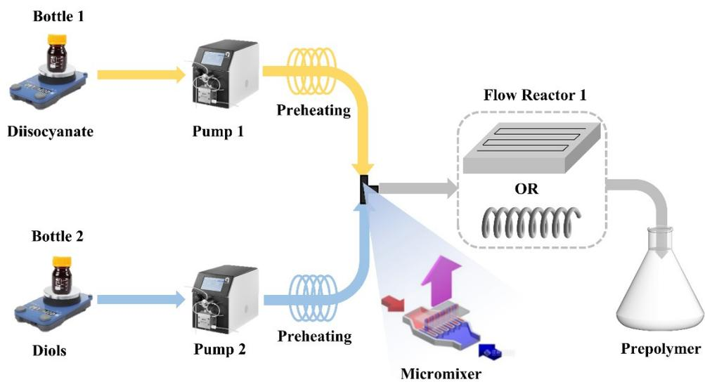
Fig. S2 Schematic diagram of prepolymer collection at the outlet of flow reactor 1.
