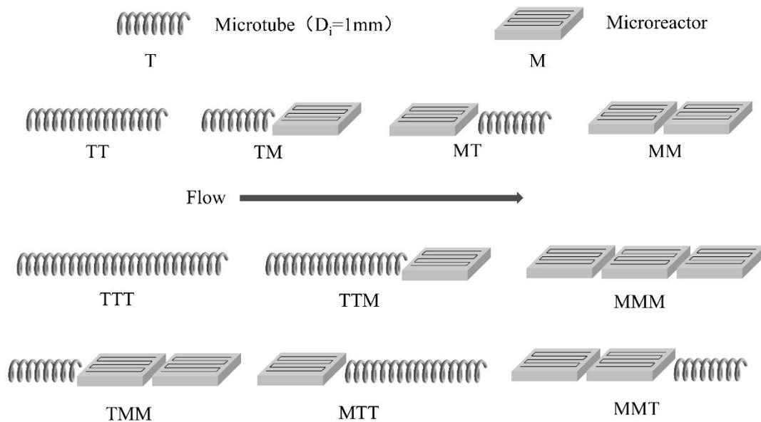
Fig. S4 Schematic diagram of different reactor configuration of microtube reactor and microreactor.
