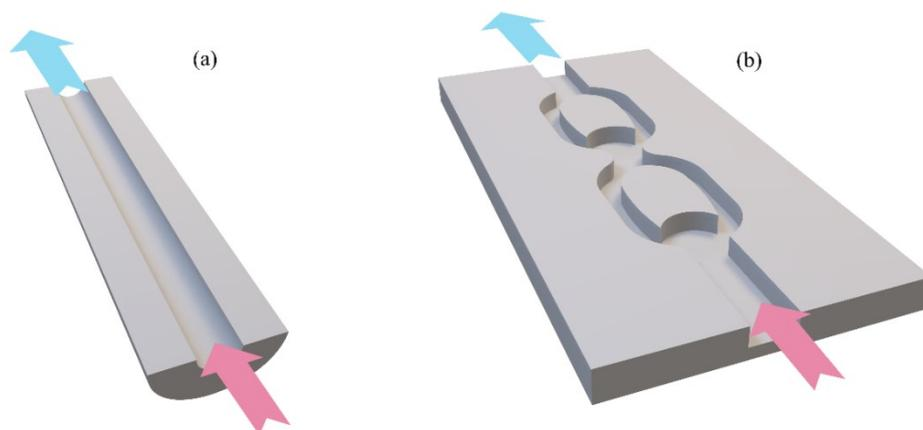
Fig. S5 Microtube reactor (a) and microreactor (b) cross section diagrams.
