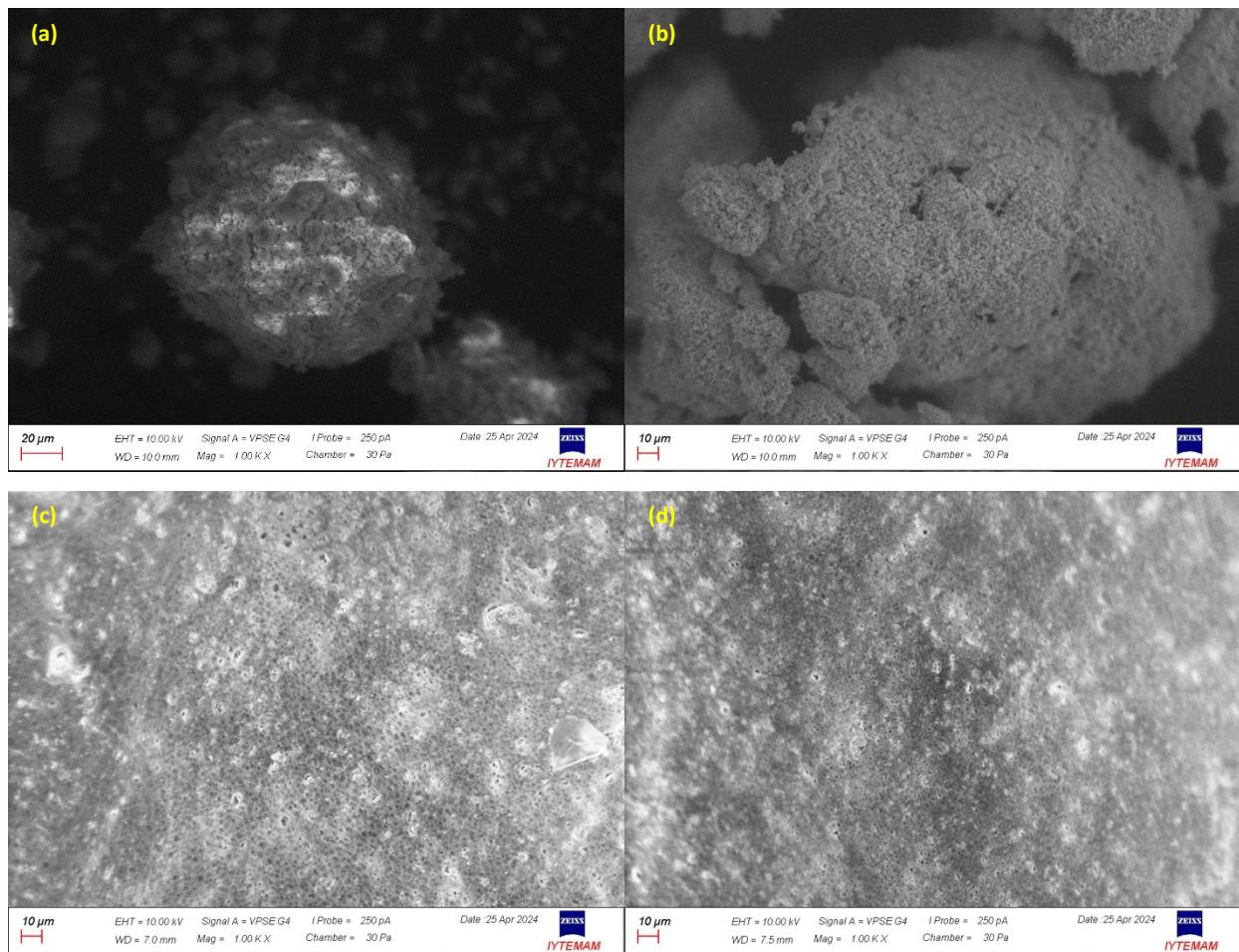
**Figure S2.** SEM images of (a) PVC/PAN, (b) LTO, (c) PVC/PAN-LTO, and (d) PVC/PAN-HTO at 1000x magnification.
