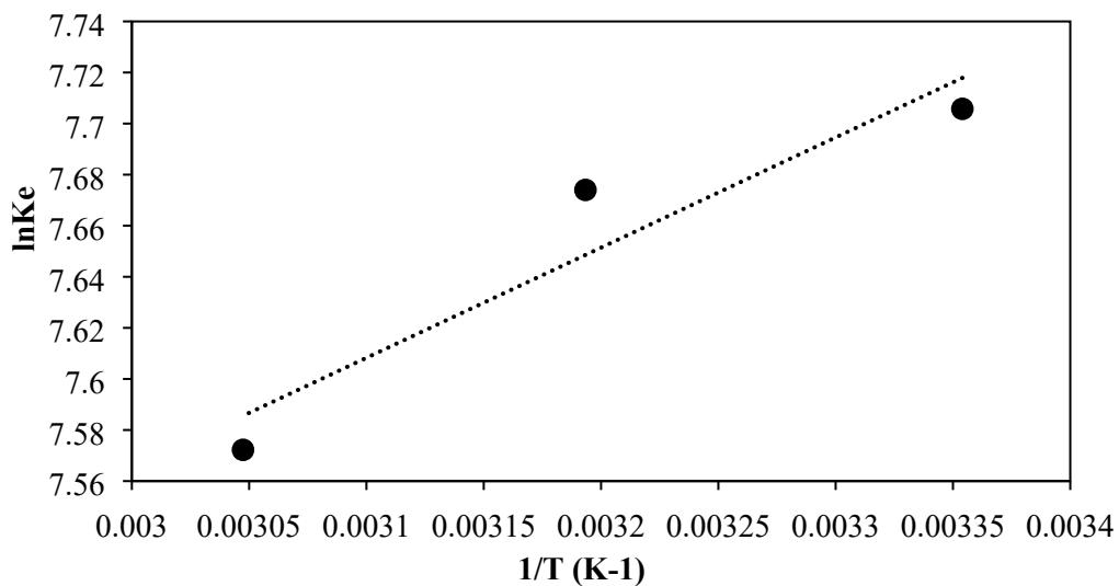
**Figure S4.**  $\ln K_e$  vs.  $1/T$  plot for thermodynamic parameter determination from van't Hoff equation.
