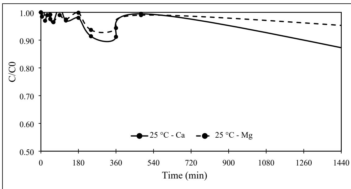
**Figure S5.** Effect contact time on competitor ions removal using PVC/PAN-HTO from geothermal water (adsorbent dose = 4 g/L, T=25°C)
