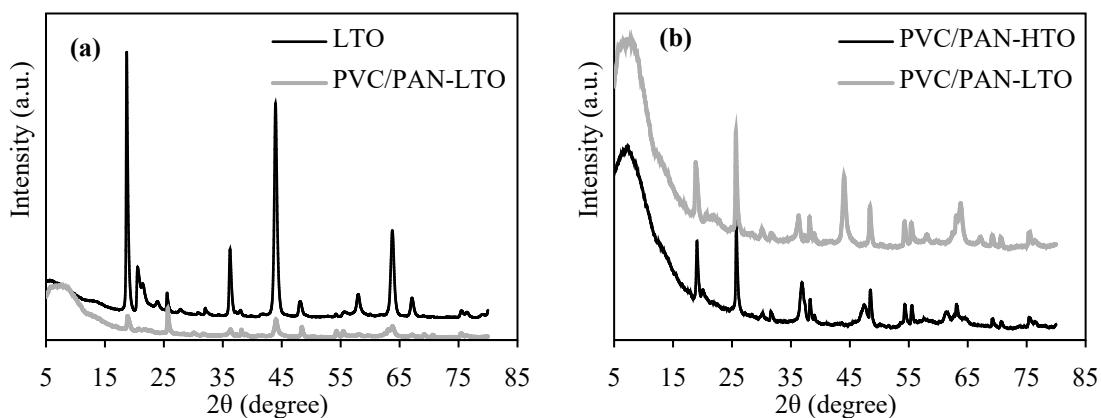
**Figure S1.** Comparison of XRD patterns of (a) LTO and PVC/PAN-LTO and (b) PVC/PAN-LTO and PVC/PAN-HTO.
