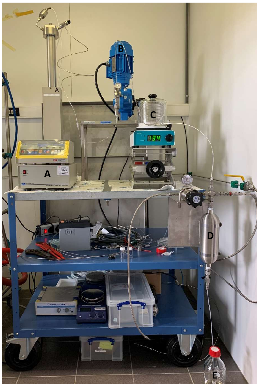
Figure S2. Photograph of the continuous flow setup (CØPE Reactor; A: pump (Teledyne Isco Hlf 500d); B: pulsator; C: reactor (Uniqsis); D: BPR; E: collection vessel).
