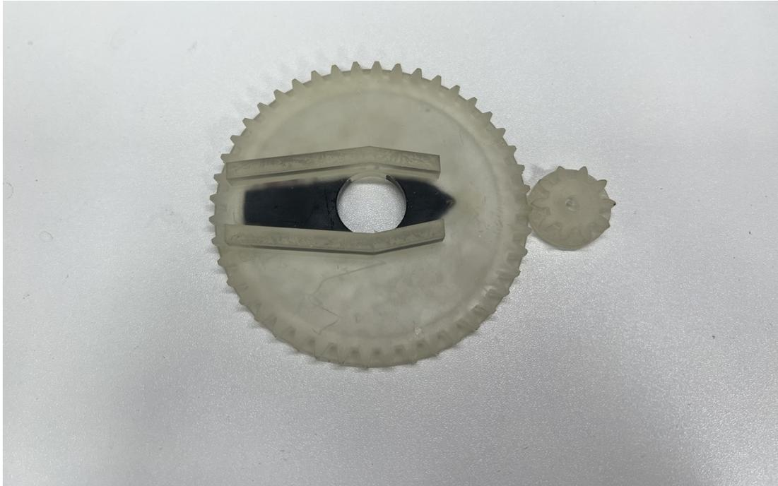
**Figure S5.** Comparison of gear sizes for five-way valves and the stepping motor.
