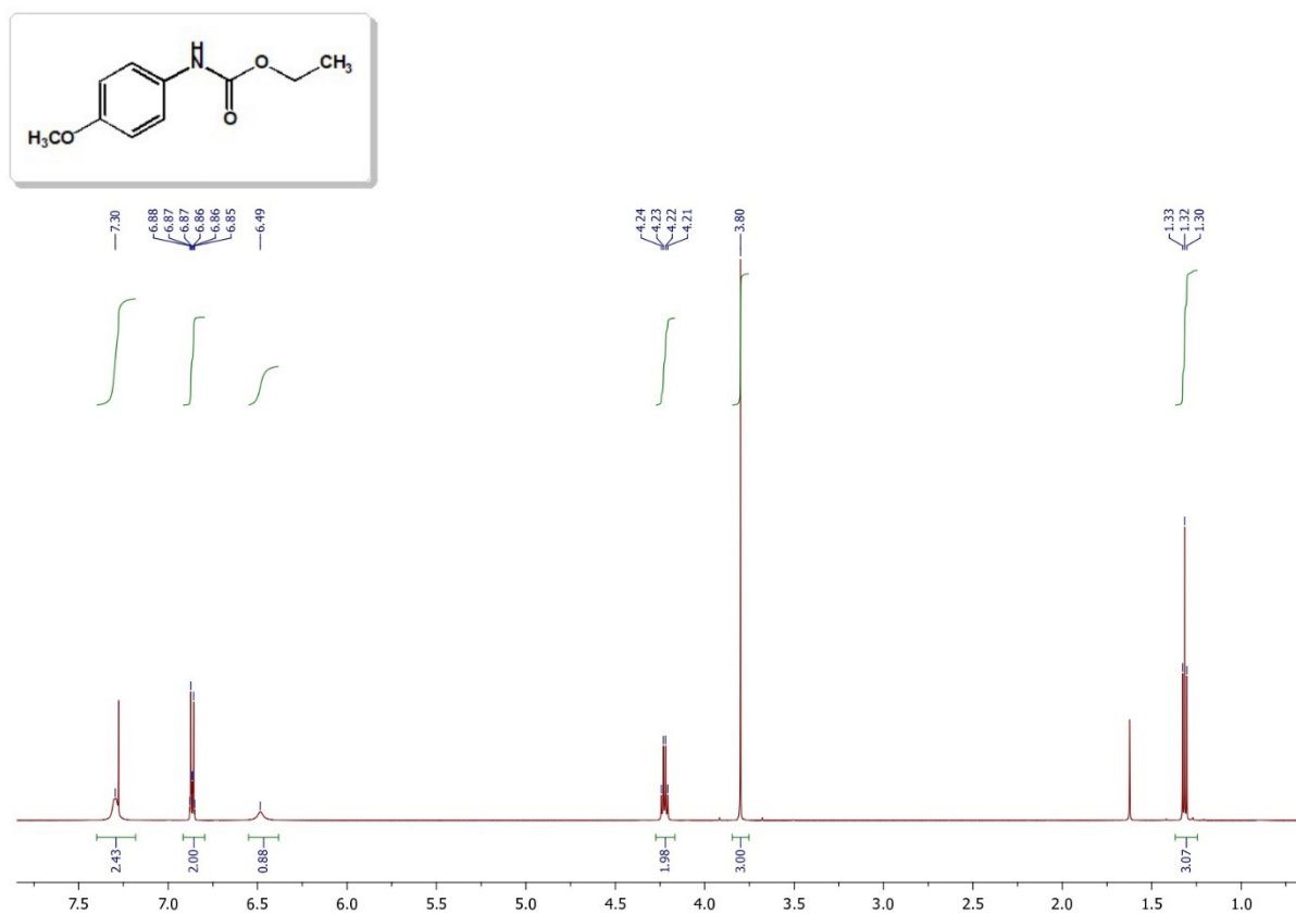
Fig. 3.13. 1 H NMR spectrum of Ethyl N-(4-methoxyphenyl)carbamate
