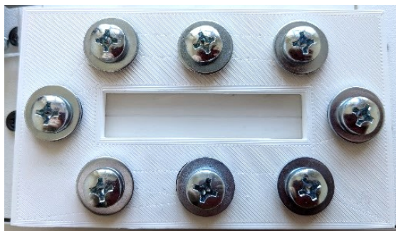
Figure S2. Image of the anssembled 3D-printed microreactor that includes the \text{TiO}_2 photocatalyst immobilized on a glass plate.
