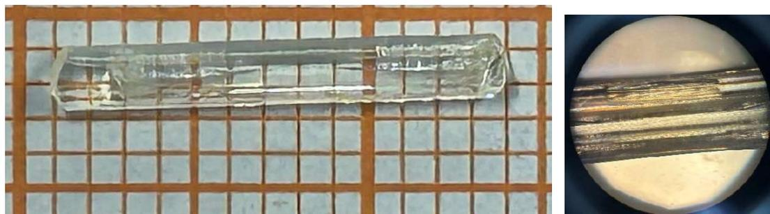
The photograph of  $\text{Cs}_3\text{Bi}_2\text{Cl}_9$  single crystals.
