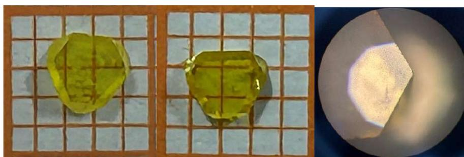
The photograph of  $\text{Cs}_2\text{AgBiCl}_6$  single crystals.
