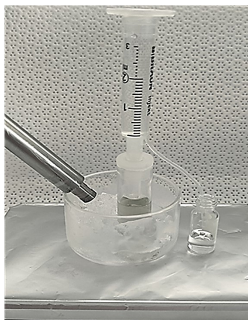
Figure S7: Scheme and picture of the employed hydrogen collection system
