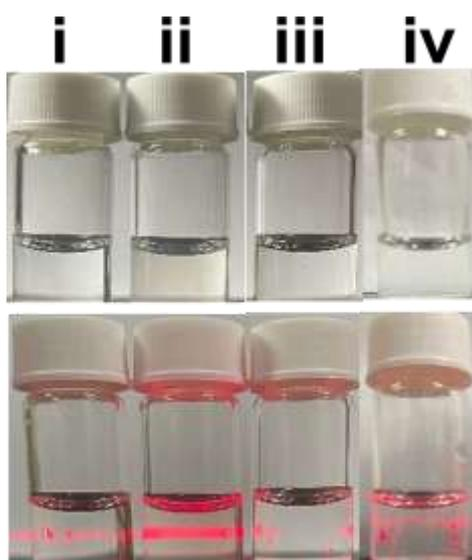
**Figure S3.** Tyndall phenomenon of the reaction solutions containing (i) Fmoc-O-phospho-L-tyrosine, (ii)  $\text{Ce}^{3+}$  and Fmoc-O-phospho-L-tyrosine, (iii)  $\text{Ce}^{3+}$  and Fmoc-L-tyrosine or (iv)  $\text{Ce}^{3+}$  and O-phospho-L-tyrosine.
