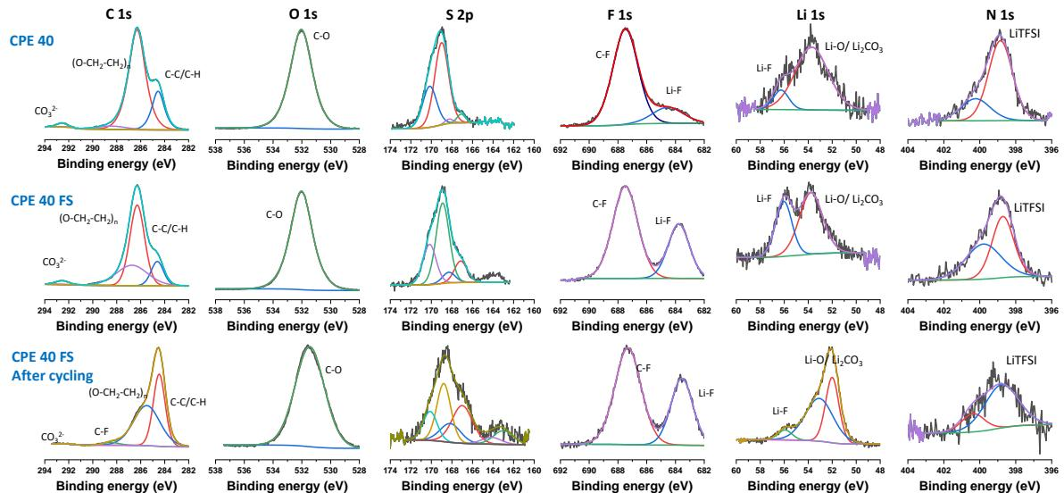
**Fig. S7.** XPS spectrum of C 1s, O 1s, S 2p, F 1s, Li 1s, and N 1s in CPE (40), CPE (40) FS, and cycled CPE (40) FS.
