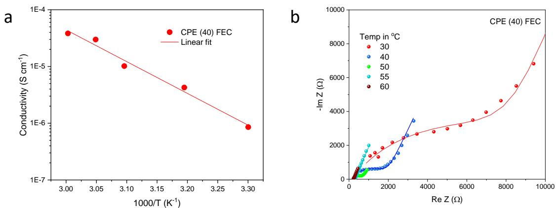
**Fig. S11.** (a)Arrhenius plot and (b) Nyquist profile of different compositions of CEP (40) FEC
