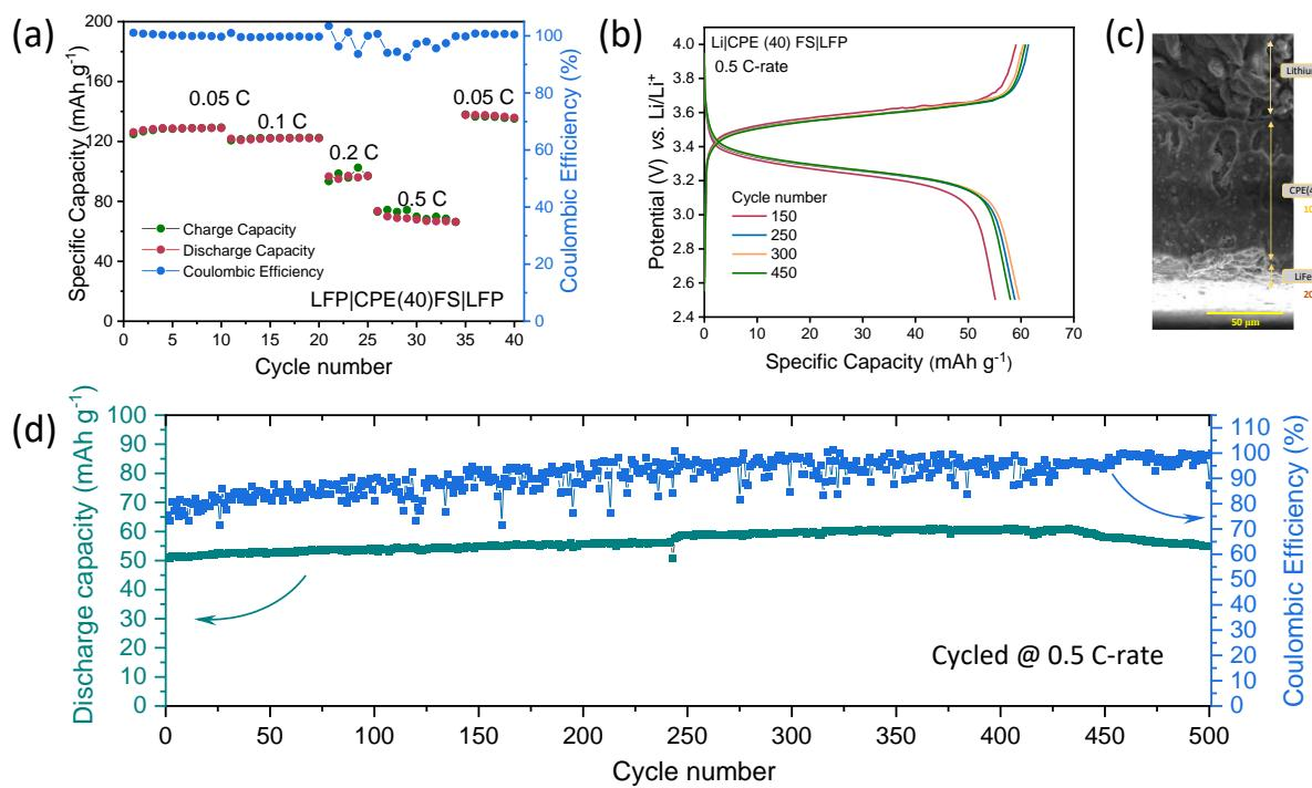
**Fig. S5.** (a) Rate capability of the full cell at 55 °C. (b) cycling profile of LFP|Li full cell cycled at 0.5 C-rate at 55 °C. (c) cross-section SEM image of the cycled cell. (d) discharge capacity and Coulombic efficiency as a function of cycle number for the LFP|Li full cell cycled at 0.5 C-rate at 55 °C.
