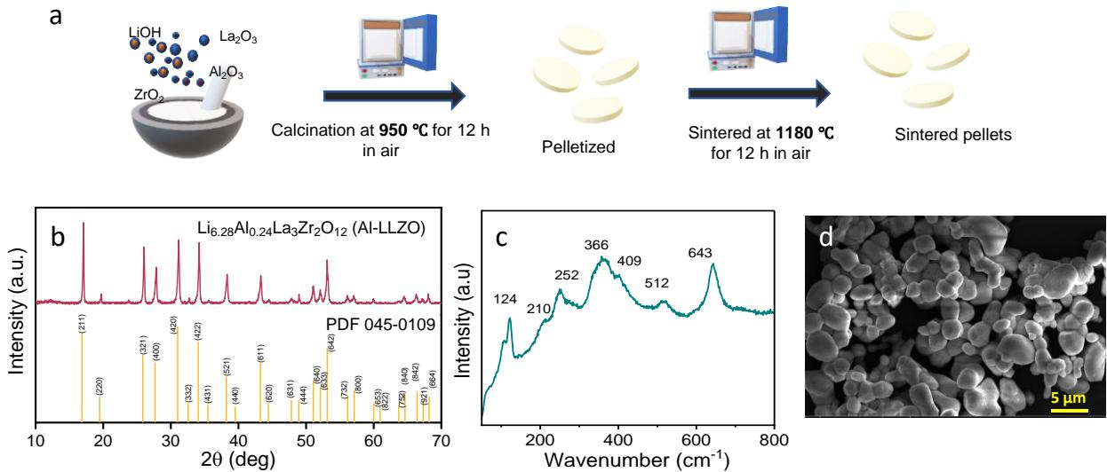
**Fig. S1.** (a) Synthesis procedure of Al-LLZO ( $\text{Li}_{6.28}\text{Al}_{0.24}\text{La}_3\text{Zr}_2\text{O}_{12}$ ), (b) XRD pattern and (c) Raman spectrum of the prepared Al-LLZO, (d) SEM image of the crushed Al-LLZO particles.
