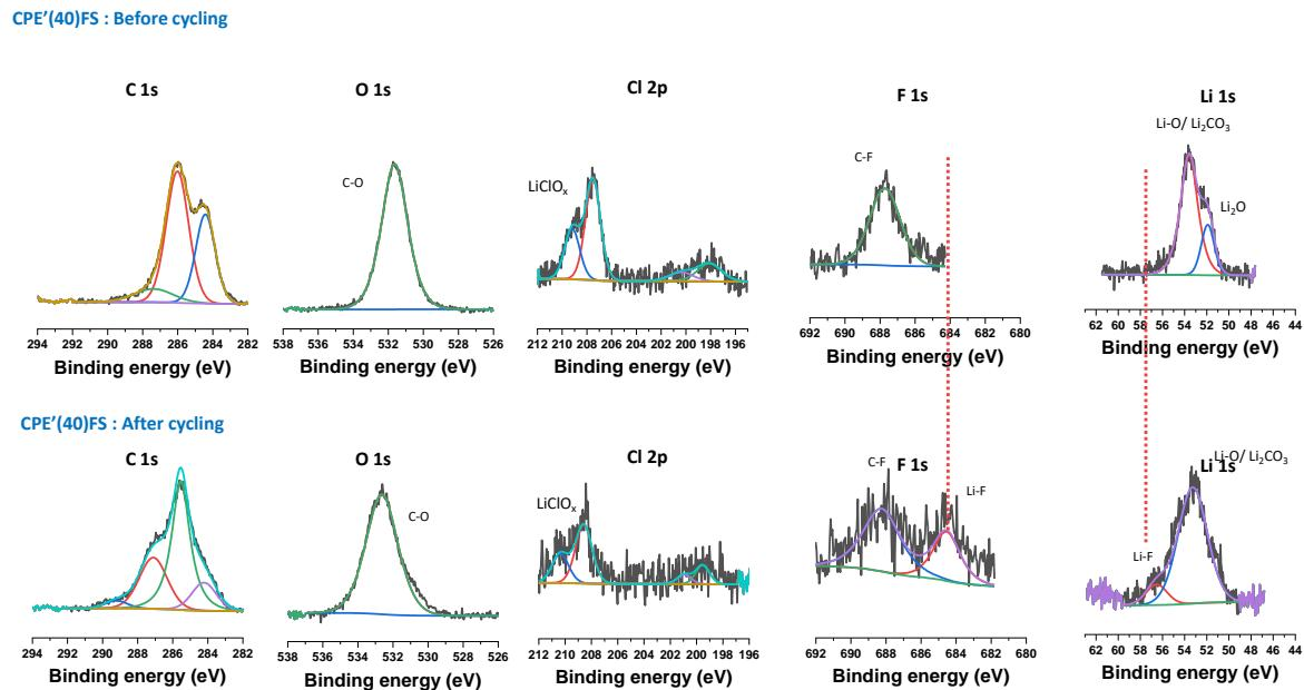
**Fig. S9.** XPS spectrum of C 1s, O 1s, Cl 2p, F 1s, and Li 1s in Al-LLZO powder obtained after washing the cycled CPE' (40) FS membrane with LiClO<sub>4</sub> salt before cycling (top), after cycling (bottom).
