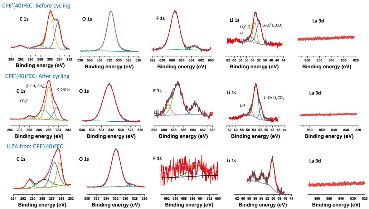
**Fig. S10.** XPS spectrum of C 1s, O 1s, S 2p, F 1s, Li 1s, and La 3d in CPE'(40) FEC before cycling, after cycling and Al-LLZO powder obtained from the cycled CPE' (40) FEC.
