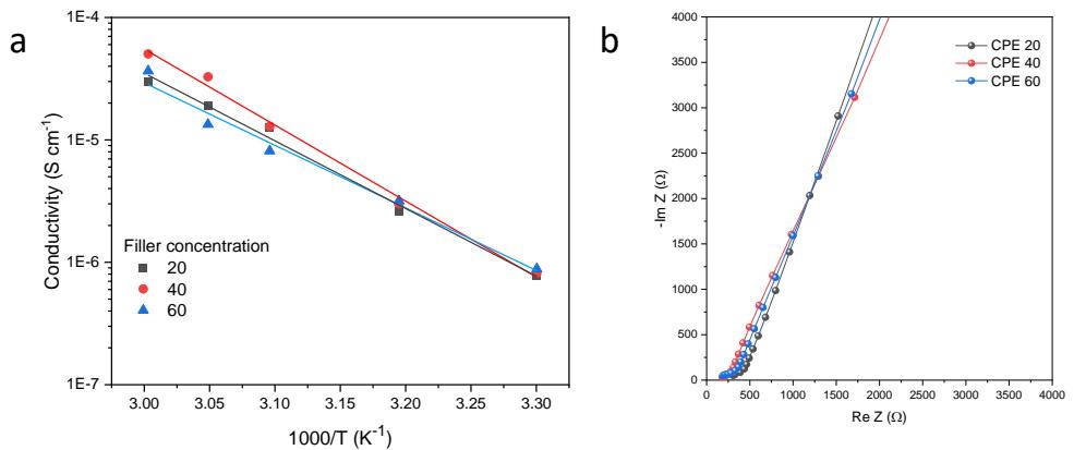
**Fig. S2.** (a) Arrhenius plot and (b) Nyquist profile of different compositions of CPEs.
