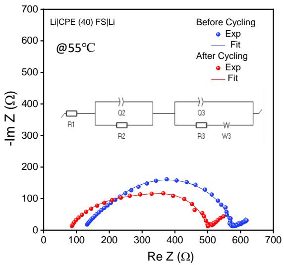
**Fig. S4.** Nyquist plot of Li|Li symmetric cell before and after long-term plating stripping studies at  $0.1 \text{ mA cm}^{-2}$
