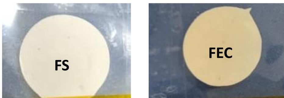
**Fig. S12.** The digital photograph of CPE (40) FS (left) and CPE (40) FEC (right) membranes
