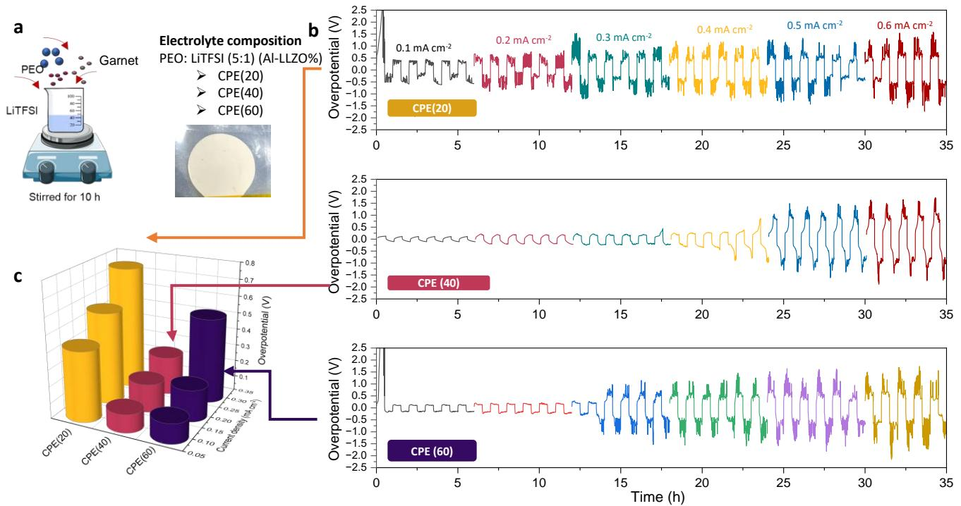
**Fig. S3.** (a) The synthesis procedure and the digital photograph of the CPE membranes, (b) Lithium stripping-plating profile of different compositions of CPEs up to  $0.6 \text{ mA cm}^{-2}$  and (c) its overpotential
