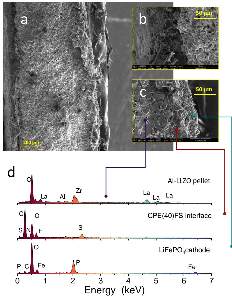
**Fig. S13 .** Post cycling SEM cross section of the full cell with CPE(40)FS as cathode interface modifier with EDS mapping
