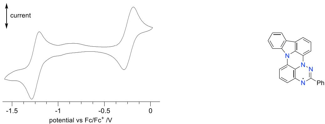
**Figure S24.** Cyclic voltammogram for **1c**.
