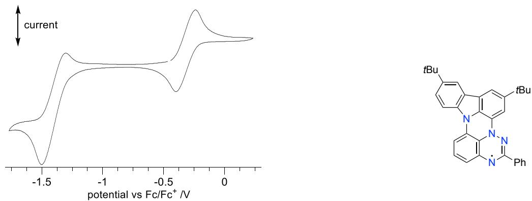
**Figure S25.** Cyclic voltammogram for **1d**.
