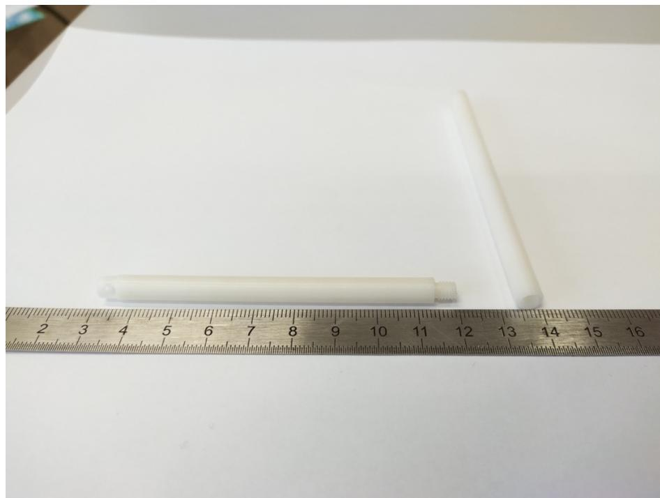
**Figure S30.** Delrin sample holder used for SQUID measurements.
