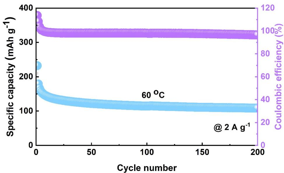
Fig.S5 The cycling performance of CityU-47 at 60 °C at the current density of 2 A g<sup>-1</sup>.
