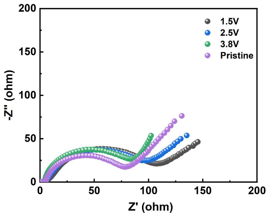
Fig.S7 The EIS plot before cycling of the sodium battery.
