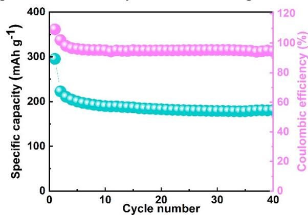
Fig.S4 The cycling performance of CityU-47 at 60 °C at the current density of 200 mA g<sup>-1</sup>.
