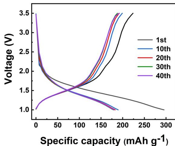
Fig.S6 The charge/discharge curves of CityU-47 at 60 °C.
