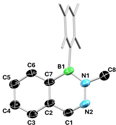
**Figure S58.** Molecular structure of compound **6Me**. Ellipsoids drawn at 50% probability. All H atoms omitted, and duryl substituent rendered as wireframe. Selected bond lengths (Å) and angles (°) of **6Me**: B1–N1 1.417(3), N1–N2 1.394(2), N2–C1 1.287(3), C1–C2 1.430(3), C2–C3 1.400(3), C3–C4 1.365(3), C4–C5 1.404(3), C5–C6 1.374(3), C6–C7 1.398(3), C7–C2 1.424(2), B1–C8 1.443(3), C1–N2–N1–B1 0.5(3).
