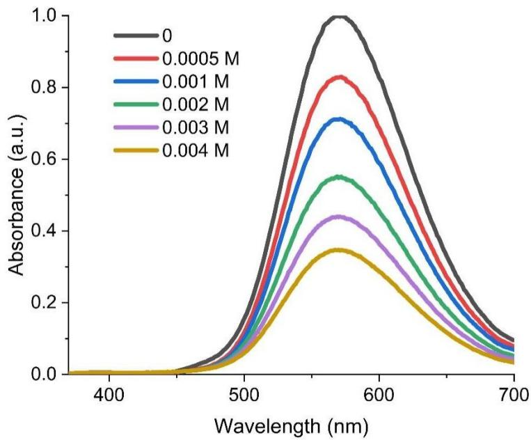
**Fig. S2.** Quenching of the **PC1** emission (0.1 mM in  $\text{CH}_3\text{CN}$ ) in the presence of **Amine-CN**.
