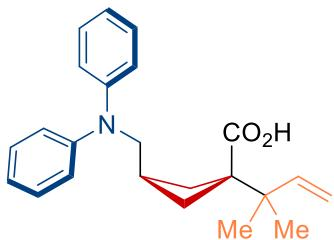
Following the general procedure, 3-methylbut-2-en-1-yl bicyclo[1.1.0]butane-1-carboxylate (66.4 mg, 0.4 mmol, 2.0 equiv.), *N*-phenyl-*N*-(trimethylsilyl)methyl)aniline (51.0 mg, 0.2 mmol, 1.0 equiv.) and Ir(dtbbpy)(ppy)<sub>2</sub>[PF<sub>6</sub>] (3.0 mg, 3.0 × 10<sup>-3</sup> mmol, 1.5 mol%), lighted in 1 W blue LED (450 nm, SYNLED) at 40 °C for 24 h. Product **17** was obtained as a colorless oil (46.8 mg, 67% yield, 1.4:1 dr).
