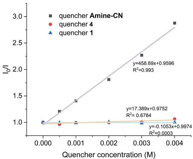
**Fig. S3.** Stern-Volmer plot for the quenching studies. Emission wavelength fixed at 571 nm. The Stern-Volmer constant ( $K_{SV}$ ) for the quenching by **Amine-CN** being  $458.7 \text{ mM}^{-1}$ .
