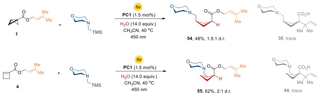
*Results:* In the presence of external water, the desired radical addition/rearrangement cascade reaction was completely inhibited. However, the aminoalkylation-protonation products **54** and **55** were detected in good yields. It supports the possible generation of  $\alpha$ -ester anion species, which are quite sensitive to the moisture.
