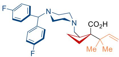
Following the general procedure, 3-methylbut-2-en-1-yl cyclobut-1-ene-1-carboxylate (33.2 mg, 0.2 mmol, 1.0 equiv.), 1-(bis(4-fluorophenyl)methyl)-4-((trimethylsilyl)methyl)piperazine (150.0 mg, 0.4 mmol, 2.0 equiv.) and Ir(dtbbpy)(ppy)<sub>2</sub>][PF<sub>6</sub>] (3.0 mg, 3.0 × 10<sup>-3</sup> mmol, 1.5 mol%), lighted in 1 W blue LED (450 nm, SYNLED) at 40 °C for 12 h. Product **46** was obtained as a white solid (47.8 mg, 51% yield, >20:1 dr).
