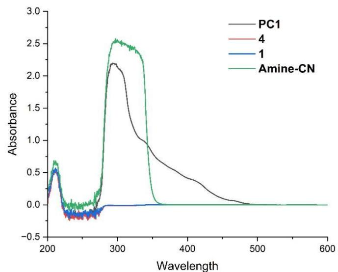
**Fig S1.** Absorption spectra of **PC1** (0.1 mM in MeCN, black line), **4** (0.5 mM in MeCN, red line), **1** (0.5 mM in MeCN, blue line), Amine-CN (0.5 mM in MeCN, green line). Absorbance is measured in arbitrary units (a.u.).
