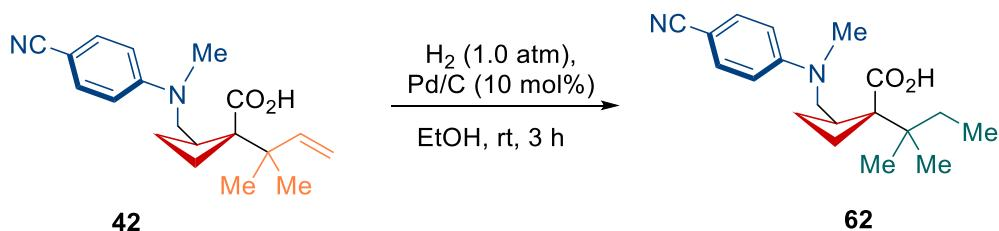
To an oven-dried 25.0 mL round-bottom flask was added **42** (62.4 mg, 0.2 mmol, 1.0 equiv., >20:1 dr), Pd/C (11.0 mg, 2.0 × 10<sup>-2</sup> mmol, 0.1 equiv.) and EtOH (5.0 mL). Then the mixture was stirred at rt for 3 h under H<sub>2</sub> atmosphere. The solvent was removed under reduced pressure and the residue was purified by flash chromatography directly on silica gel (petroleum ether/ethyl acetate 3:1) to obtain product **62** as a colorless oil (47.1 mg, 75% yield, >20:1 dr).
