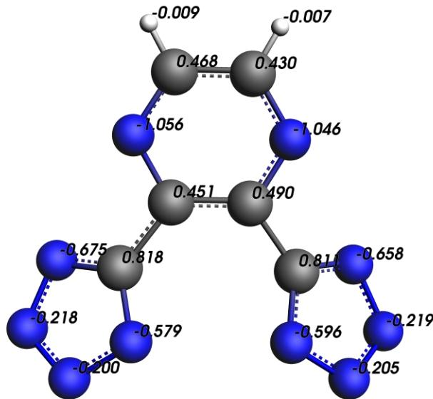
**Figure S6.2** The Quantum Theory of Atoms in Molecules (QTAIM) charge of dtp<sup>2-</sup> before coordinating with Pu<sup>3+</sup>. This dtp<sup>2-</sup> is coordinated with Pu<sup>3+</sup> through two nitrogen atoms from all tetrazolate.
