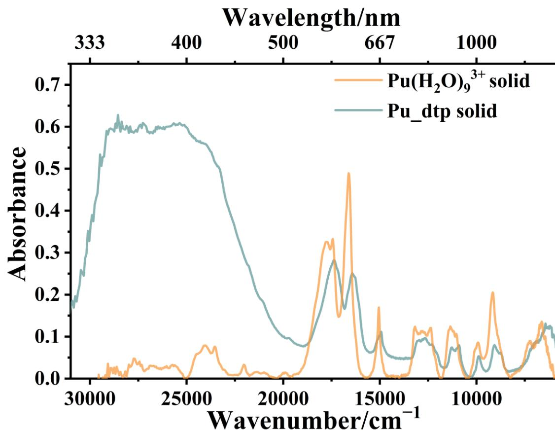
**Figure S5.1** Solid state UV-vis-NIR spectra of Pu\_dtp (blue) and  $[Pu(H_2O)_9]^{3+}$ <sup>3</sup> (brown) at room temperature.
