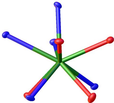
**Figure S3.1** A view of the local coordination environment (spherical capped square antiprismatic geometry with a deviation value of 0.928, from the analysis via SHAPE software<sup>1,2</sup>) of the Pu<sup>3+</sup> cation within **Pu\_dtp** from OLEX2.
