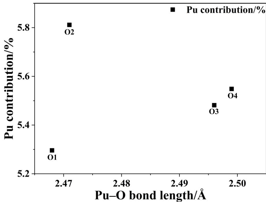
**Figure S7.2.** Plutonium contribution to selected NLMOs of average  $\alpha + \beta$  spin Pu–H<sub>2</sub>O in Pu\_dtp.
