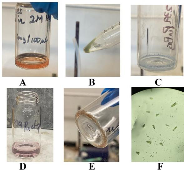
**Figure S2.1.** A. Stock solution of  $^{239}\text{Pu}^{\text{n}+}$  (1 mg/0.1mL). B. Pellet of  $^{239}\text{Pu}(\text{OH})_4$  after centrifugation. C.  $^{239}\text{PuBr}_3 \cdot \text{nH}_2\text{O}$ . D. Reaction picture. E. Crystals of **Pu\_dtp** grown from aqueous solution. F. Crystals of **Pu\_dtp** used for single-crystal X-ray diffraction and solid-state UV-vis-NIR spectroscopy.
