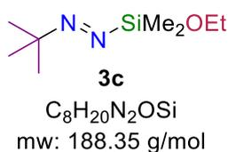
$^1H$  NMR (300 MHz,  $CDCl_3$ ):  $\delta/ppm = 3.89$  (q,  $J = 7.0$  Hz, 2H), 1.24 (t,  $J = 7.0$  Hz, 3H), 1.17 (s, 9H), 0.23 (s, 6H).  $^{13}C\{^1H\}$  NMR (75 MHz,  $CDCl_3$ ):  $\delta/ppm = 74.5, 59.4, 26.0, 18.6, -4.3$ .  $^1H/^{29}Si$  HMQC NMR (300/60 MHz,  $CDCl_3$ ):  $\delta/ppm = 0.24/-3.0$ . HRMS (ESI)  $m/z$ :  $[M+H]^+$  Calcd for  $C_8H_{20}N_2OSiH$  189.1418. Found 18.1415
