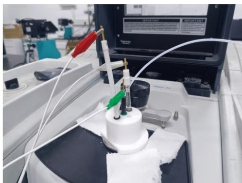
**Figure S18.** Device photo of in-situ FTIR.
