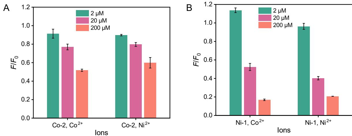
**Figure S4.** The response of aptamers (A) Co-2 and (B) Ni-1 to 2  $\mu\text{M}$ , 20  $\mu\text{M}$  and 200  $\mu\text{M}$   $\text{Co}^{2+}$  or  $\text{Ni}^{2+}$  (Aptamers: 0.5  $\mu\text{M}$ , ThT: 1  $\mu\text{M}$ , buffer: 10 mM MES pH 6, 100 mM NaCl, 2 mM  $\text{MgCl}_2$ ).  $F_0$  and  $F$  denote the fluorescence before and after adding ions, respectively.
