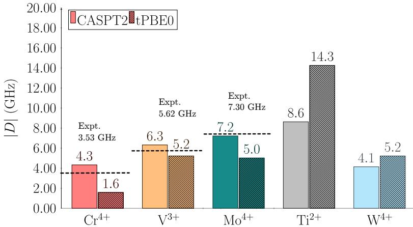
Figure S20: Calculated axial parameter ( $|D|$ ) with the CASPT2 (solid bar) and tPBE0 (striped bar) methods for the  $\text{Cr}(o\text{-tol})_4$  (red),  $\text{V}(o\text{-tol})_4^-$  (orange),  $\text{Mo}(o\text{-tol})_4$  (teal),  $\text{Ti}(o\text{-tol})_4^{2-}$  (gray), and  $\text{W}(o\text{-tol})_4$  (cyan) complexes using (2,5) active space. The values are in GHz. Dashed lines correspond to experimental data from references 1 and 2.
