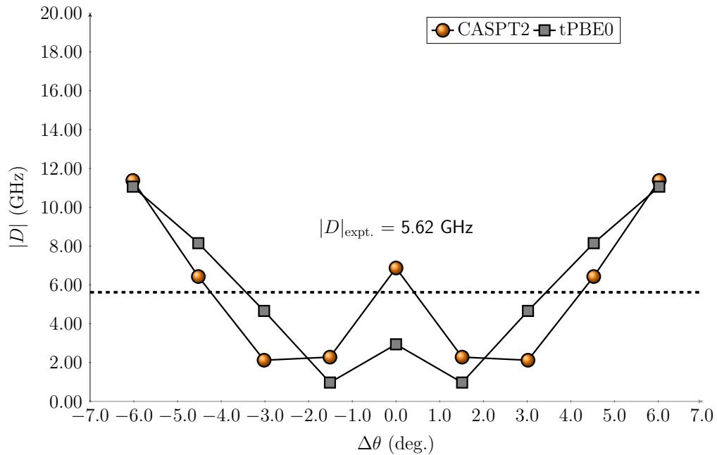
Figure S39: Zero-field splitting parameters computed with CASPT2 and tPBE0 methods for the  $V(o\text{-tol})_4^-$  complex considering the C–V–C scissoring normal mode. The equilibrium bond angle is  $\theta = 105.2^\circ$ .
