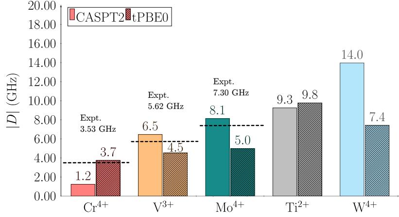
Figure S21: Calculated axial parameter ( $|D|$ ) with the CASPT2 (solid bar) and tPBE0 (striped bar) methods for the  $\text{Cr}(o\text{-tol})_4$  (red),  $\text{V}(o\text{-tol})_4^-$  (orange),  $\text{Mo}(o\text{-tol})_4$  (teal),  $\text{Ti}(o\text{-tol})_4^{2-}$  (gray), and  $\text{W}(o\text{-tol})_4$  (cyan) complexes using (2,10) active space. The values are in GHz. Dashed lines correspond to experimental data from references 1 and 2.
