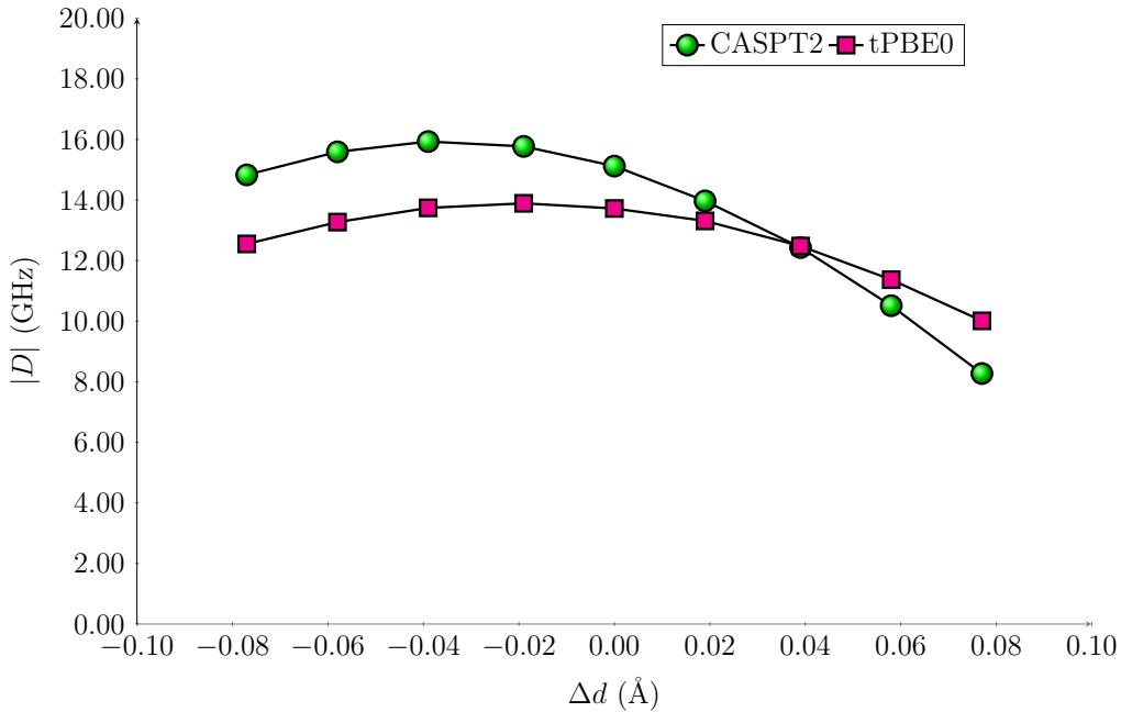
Figure S40: CASPT2 and tPBE0 axial parameter ( $|D|$ ) of  $\text{Ti}(o\text{-tol})_4^{2-}$  complex for the Ti–C symmetric stretching normal mode. The equilibrium bond distance is  $d = 2.16 \text{ \AA}$ .
