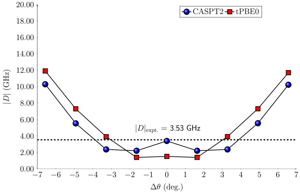
Figure S37: CASPT2 and tPBE0 axial parameter ( $|D|$ ) of  $\text{Cr}(o\text{-tol})_4$  complex for the C–Cr–C scissoring normal mode. The equilibrium bond angle is  $\theta = 104.9^\circ$ .
