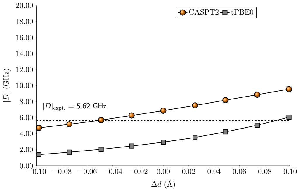
Figure S38: CASPT2 and tPBE0 axial parameter ( $|D|$ ) of  $V(o\text{-tol})_4^-$  complex for the V–C symmetric stretching normal mode. The equilibrium bond distance is  $d = 2.07 \text{ \AA}$ .
