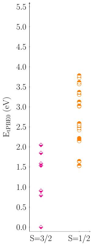
Figure S18: Relative energies of  $\text{Co}(o\text{-tol})_4^{2-}$  molecule computed with the tPBE0 method for the (13,13) active spaces. The magenta half-filled rhombus corresponds to quartet states and the orange half-filled circles to doublet states.
