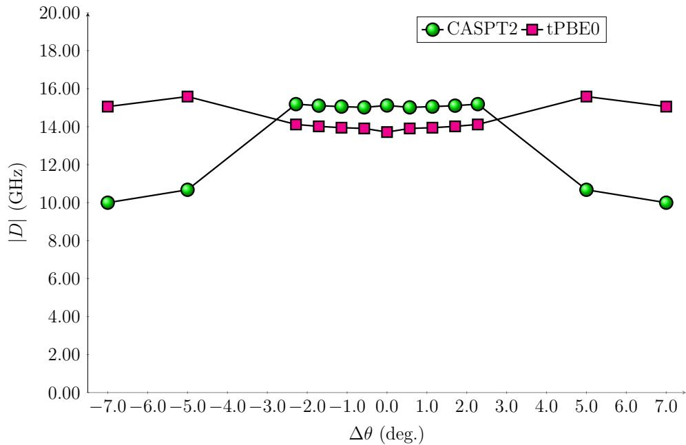
Figure S41: CASPT2 and tPBE0 axial parameter ( $|D|$ ) of  $\text{Ti}(o\text{-tol})_4^{2-}$  complex for the C–Ti–C scissoring normal mode. The equilibrium bond angle is  $\theta = 106.0^\circ$ .
