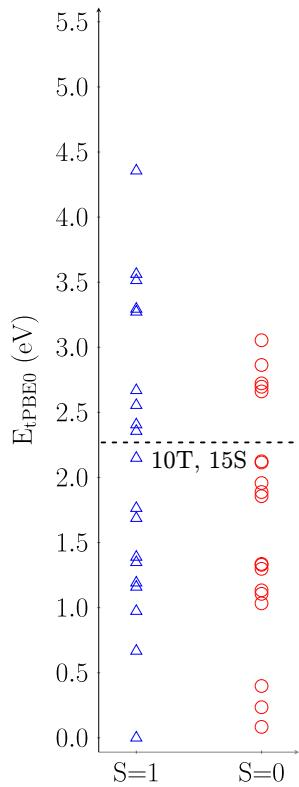
Figure S15: Relative energies of  $\text{Ti}(o\text{-tol})_4^{2-}$  molecule computed with the tPBE0 method for the (10,15) active spaces. The blue triangles correspond to triplet states and the red circles to singlet states.
