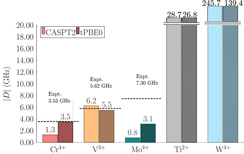
Figure S22: Calculated axial parameter ( $|D|$ ) with the CASPT2 (solid bar) and tPBE0 (striped bar) methods for the  $\text{Cr}(o\text{-tol})_4$  (red),  $\text{V}(o\text{-tol})_4^-$  (orange),  $\text{Mo}(o\text{-tol})_4$  (teal),  $\text{Ti}(o\text{-tol})_4^{2-}$  (gray), and  $\text{W}(o\text{-tol})_4$  (cyan) complexes using (8,8) active space. The values are in GHz. Dashed lines correspond to experimental data from references 1 and 2.
