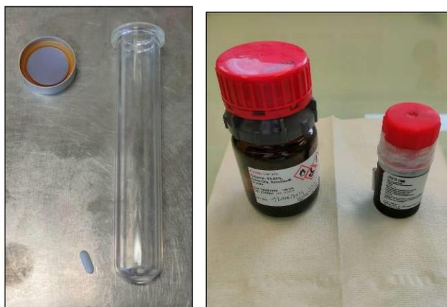
Figure S14 : Glassware used and reagents for all exchange experiments, 5 mL microwave tube with stirring bar and seal.
