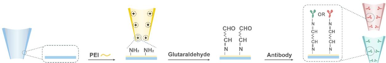
**Figure S16.** The fabrication procedure of antibody-modified nanopipettes.
