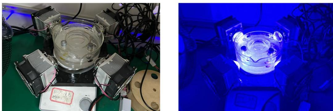
Figure S5. Picture of 30 W 450 nm irradiator
