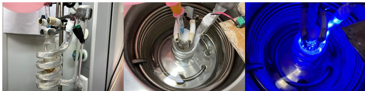
(LED: 460-465nm, 0.2W per 5050 LED lamp bead)
