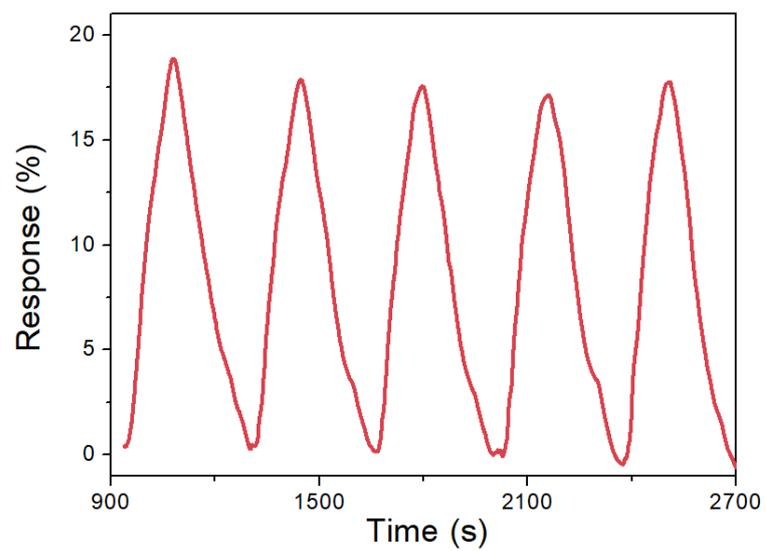
**Figure S15.** Reproducibility of the 7D-C<sub>60</sub> complex for 1 ppm NO<sub>2</sub>.
