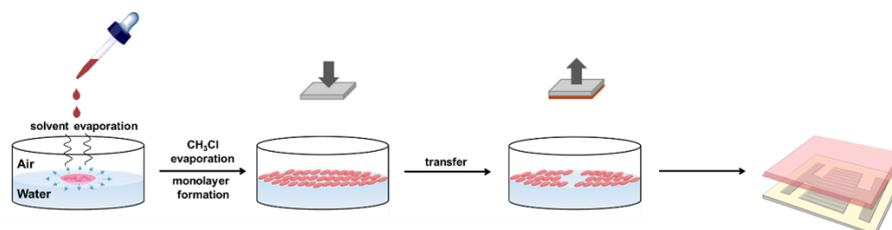
**Figure S12.** The fabrication of film electrodes by QLS method.
