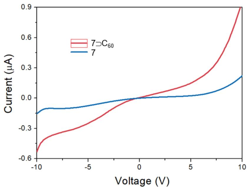
**Figure S13.**  $I$ - $V$  curves of the  $7\supset C_{60}$  complex and **7**
