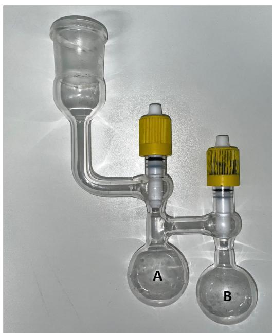
**Figure S1.** Picture of the double bulb distillation apparatus used for the volatiles transfer experiment.
