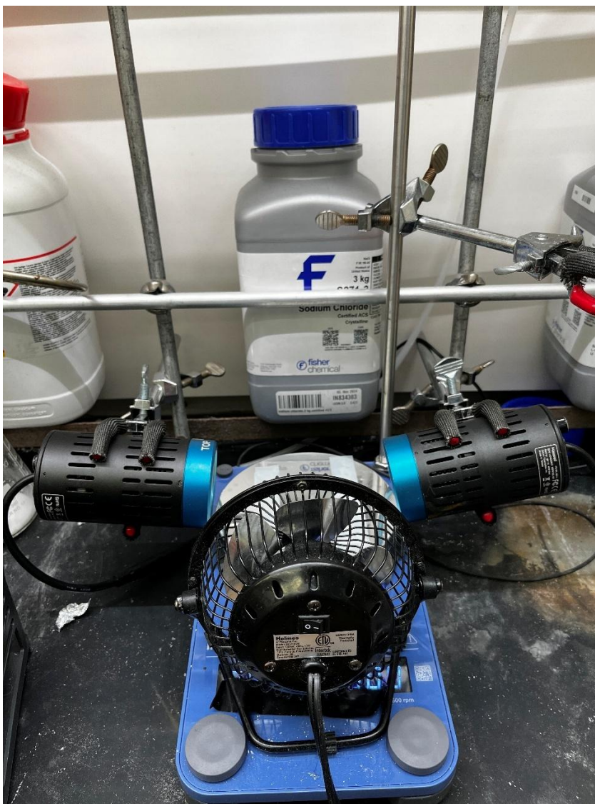
Figure S1: Photochemical setup for visible-light-mediated synthesis of 2-oxetanes.
