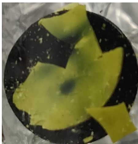
Figure S8 A photograph of 1 after XPS measurement, showing where the sample has turned blue at the point of measurement.
