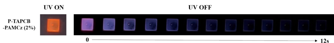
Figure S32. Photographs of p-TAPCB-PAMCz (2%) under 300 nm UV light and the afterglow after turning off the UV light.
